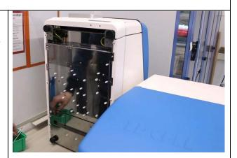
**2.** Remove the two screws on the underside of the device.
