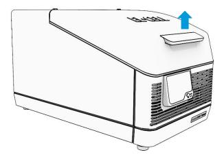
Pull the handle to open the lid of the cell chamber. When closing, make sure that you hear the lid click into place.
